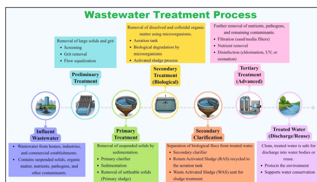
Figure 1: Step-wise demonstration of wastewater treatment
